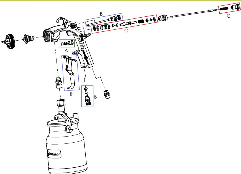
**Maintenance kit FStart Pressure / Suction 129.756.902 composed of:**
