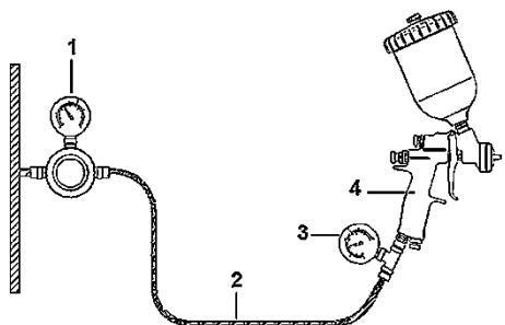
3 - P 1 : Pressure measured at the gun handle during the operating (air needles open)
