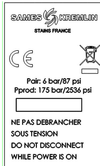
Marking label on the fluid module (fluid module located outside the spray booth in a safe area)
