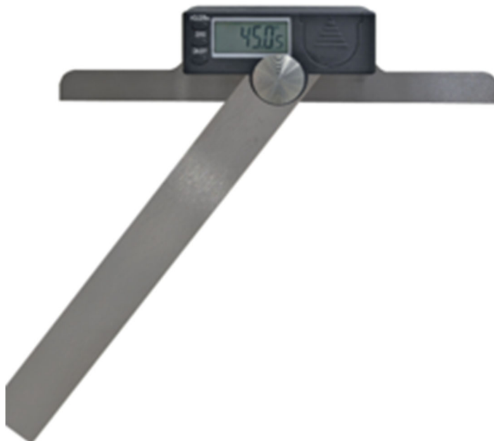
Fig. 11-2: Angle meter for adjusting the two-joint rockers
