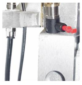
**Direct piloting** allows the user to connect the air motor reversing system (called a pilot) to an independent source of pressure. This allows the user to start the motor at a supply pressure of approximately 0.5 bar or to use the pilot pressure to control the starting and stopping of the motor.
