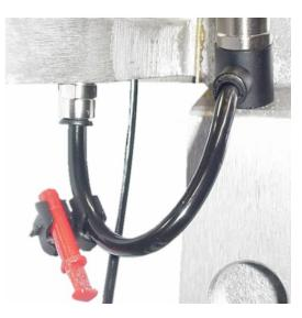
All factory assembled motors are wired in **standard control**. This means that the air motor reversing system (called pilot) is connected to the same pressure as the main motor supply. In this case, the starting threshold of the motor is approximately 1.5 bar / 21.7 psi.
