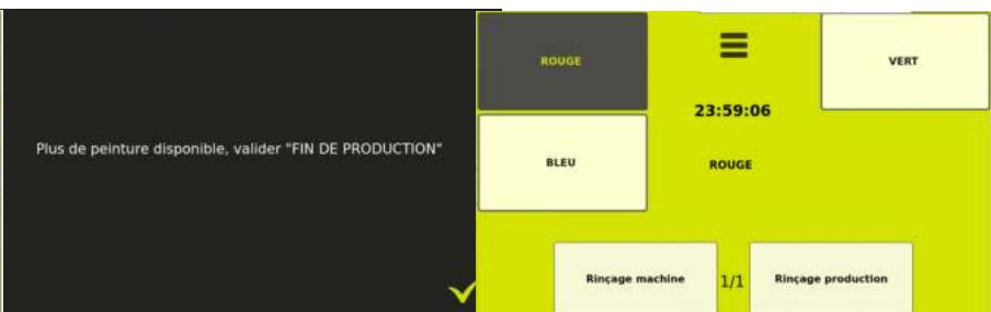
As soon as one of the volumes on a circuit is empty, the circuit supply valve closes, the volume displays 0cc and is written in red.
