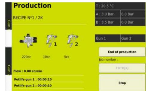
As the application progresses, the volume of the machine first decreases, regardless of the gun used. Once this volume has been fully used, it changes to 0cc and is written in red.
