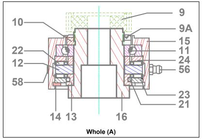
Change the whole (A). Reinstall the receiver pinion (9), the 2 pins (8), the washer (28) and the 2 screws (29).
