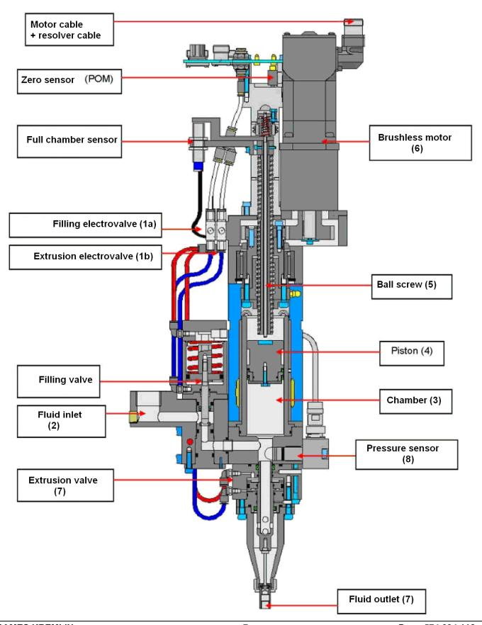
The dispensing system consists of 3 actuators :
