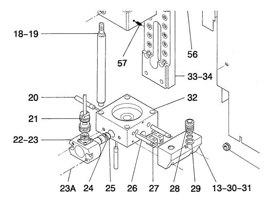
Remove the inlet valve and the outlet valve of the proportioning system.
