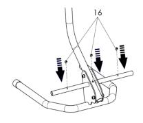
✓ Install the 3 screws (16) by means of a 4 mm BTR wrench.
