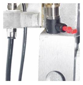
**Direct piloting** allows the user to connect the air motor reversing system (called a pilot) to an independent source of pressure. This allows the user to start the motor at a supply pressure of approximately 0.5 bar or to use the pilot pressure to control the starting and stopping of the motor.
