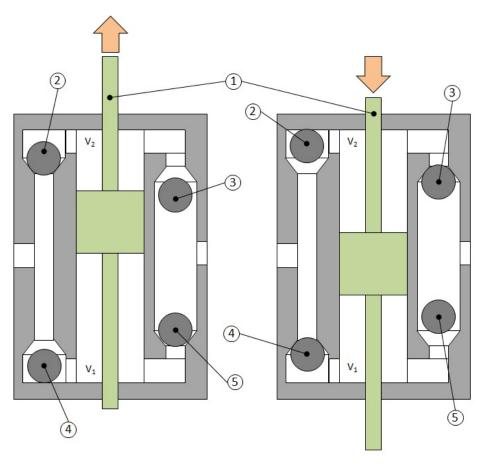
When the piston (1) rises, check-valves 2 and 5 close, while check-valves 3 and 4 open. The piston (1) expels the product from the upper chamber (V2) to the outside and sucks the product to fill the lower chamber (V1).
