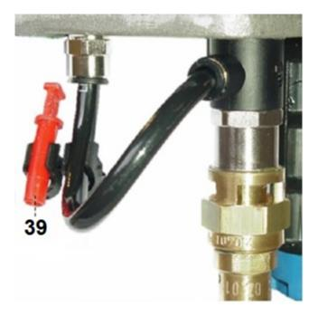
All factory assembled motors are wired in standard control. This means that the pneumatic motor reversing system (called pilot) is connected to the same pressure as the main motor supply. In this case, the starting threshold of the motor is approximately 21.7 psi. (1,5 bar).
