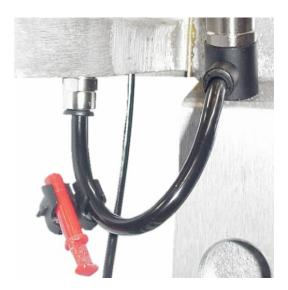
All factory assembled motors are wired in **standard control**. This means that the air motor reversing system (called pilot) is connected to the same pressure as the main motor supply. In this case, the starting threshold of the motor is approximately 1.5 bar / 21.7 psi.
