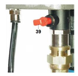
**Direct piloting** allows the user to connect the pneumatic motor reversing system (called pilot) to an independent pressure source. This allows the user to start the motor at a supply pressure of approximately 7.25 psi (0.5 bar) or to use the pilot pressure to control the starting and stopping of the motor.
