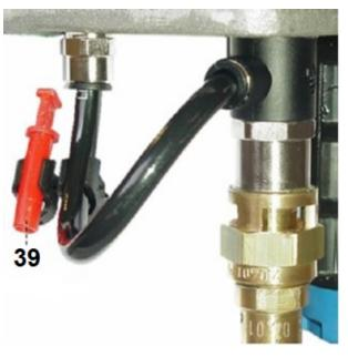
All factory assembled motors are wired in **standard control**. This means that the pneumatic motor reversing system (called pilot) is connected to the same pressure as the main motor supply. In this case, the starting threshold of the motor is approximately 21.7 psi. (1,5 bar).
