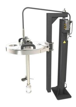
This elevator-agitator for 20-40 drums features a double-effect jack for a fast lift of a stainless steel cover fitted for a quick material drum change. The cover is equipped with a motorized agitator fitted with blades for low viscosity materials and a full stainless steel rod. The elevator is coming on a large fixing plate which makes it very stable and easy to install in paint kitchens, existing installations or an essential component of new installations
