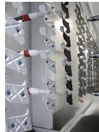
Standard installation with MCR panel and two reciprocators
