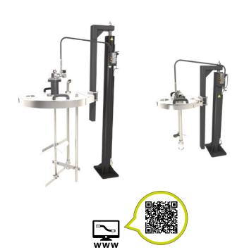
This elevator-agitator for 20-40 to 200 L drums features a double-effect jack for a fast lift of a stainless steel cover fitted for a quick material drum change. The cover is equipped with a motorized agitator fitted with blades for low viscosity materials and a full stainless steel rod.
