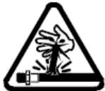
When working with high pressure application equipment, special care is required. Fluid lines may burst from excessive pressures. This increases the risk of a material injection wound under the skin.
