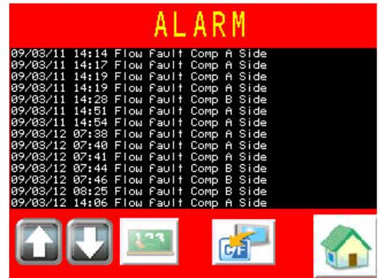
The most recent fault is displayed at the bottom of the list. The operator can use the up and down icons to navigate through the list. Refer to the trouble shooting guide in the user manual for additional help with alarms. The table below contains a brief description of the alarm message. See section regarding alarm troubleshooting guide for in depth information regarding the alarms.
