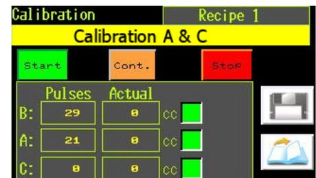
The user is display a confirmation screen which allows the user to review the new parameters and compare them to the old values. Large shift in values should not be accepted without reviewing the information for possible errors. Repeat the calibration if doubt exist.
