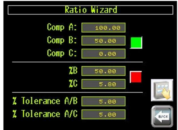
The wizard also calculates the Min/Max ratio tolerance parameters. The operator can adjust the percentage of acceptable tolerance for each ratio calculation. When the load icon is selected the parameters on screen 2/10 are updated.
