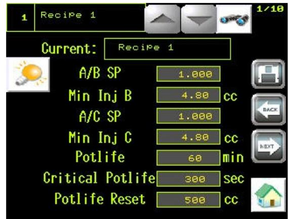
The main screen displays the Recipe Name and Index number. The index number is used in the consumption data export for later identification.
