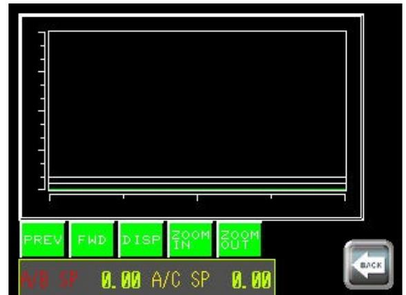
This screen shows the A/B and A/C set points in green and the calculated valves in red. The operator is allowed to move backwards in time, viewing the entire paint cycle by pressing the green
