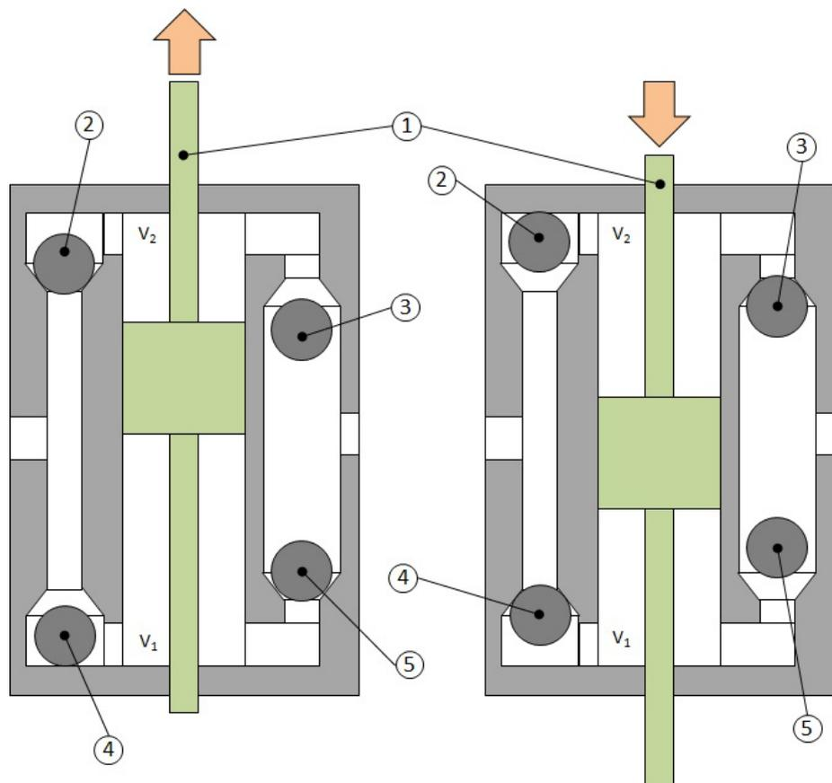
When the piston (1) rises, check-valves 2 and 5 close, while check-valves 3 and 4 open. The piston (1) expels the product from the upper chamber (V<sub>2</sub>) to the outside and sucks the product to fill the lower chamber (V<sub>1</sub>).
