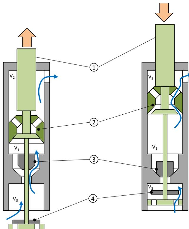
When the piston (1) rises, the upper flap (2) closes, the lower flap (3) opens and the pallet (4) closes. The piston (1) expels the product from the upper chamber (V2) to the outside and sucks the product to fill the lower chamber (V1). The pallet pushes the product into the pump foot (V3)
